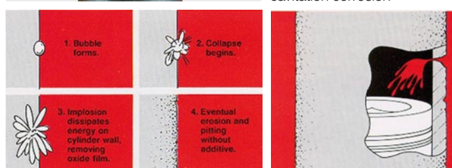
Example of cavitation corrosion
